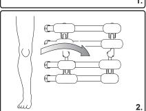
2. Position brace in a flat position as shown. Set leg over brace centered approximately between both struts.
