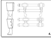
**4.** Position brace in a flat position as shown. Set leg over brace centered approximately between both struts.
