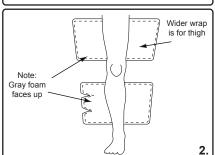
2. Remove, unroll, and lay flat each of the two soft good foam wraps with the gray foam facing up. The wider wrap is for the thigh and the narrower wrap with the saw-tooth side cut is for the calf. Position the leg over the foam wraps approximately in the center.
